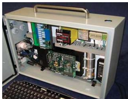
Field Control Cabinet
